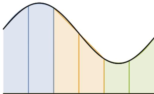
**Figure:** Simpson's rule can be seen as piecewise quadratic interpolation between the nodes  $(x_{i-1}, f(x_{i-1}))$ ,  $(x_i, f(x_i))$ , and  $(x_{i+1}, f(x_{i+1}))$  for  $i \in \{1, 3, 5, \dots\}$ .
