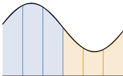
**Figure:** Simpson's  $\frac{3}{8}$  rule can be seen as piecewise cubic interpolation between the nodes  $(x_{i-1}, f(x_{i-1}))$ ,  $(x_i, f(x_i))$ ,  $(x_{i+1}, f(x_{i+1}))$ , and  $(x_{i+2}, f(x_{i+2}))$  for  $i \in \{1, 4, 7, \dots\}$ .
