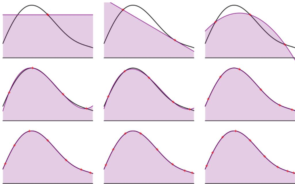
Gaussian quadrature of a function  $f$  in  $[-1, 1]$ . For the  $n$ -point rule, the quadrature nodes  $(x_i)_{i=1}^n$  are taken as the roots of the Legendre polynomial  $P_n$ . The approximation of the integral is the signed area trapped by the Lagrange interpolating polynomial of  $f$ , when interpolation is carried out with respect to the Legendre roots  $x_1 < \dots < x_n$ .
